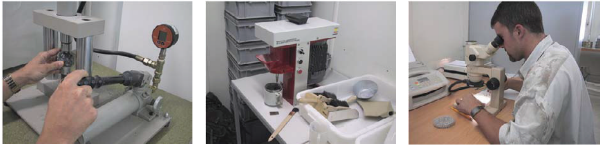
Figure 4. Left: point-Load device; middle: breakability and abrasivity machinery; right: microscopy analysis
