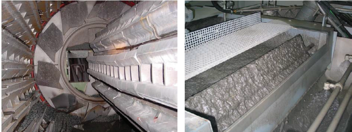
Figure 2. Left: grain rounding machine (Hurricane); right: flotation facility
